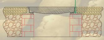
Wrong way of installation where frame is partially supported at the bottom
